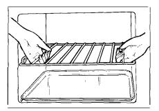
To position the DOUBLE DUTY<sup>™</sup> shelf, tip the back slightly and fit the shelf support guides onto the support guides located on each side of the oven in the rear.
